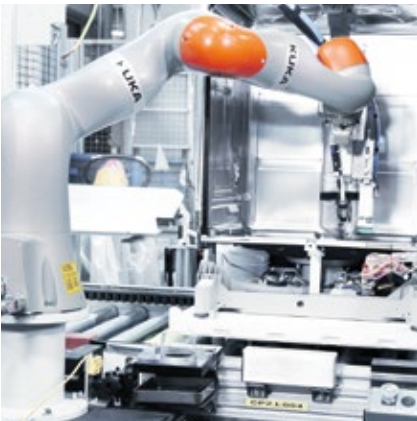
Thanks to its sensory capabilities, the LBR iiwa independently and reliably moves to the exact position of the workpiece to perform sensitive assembly tasks.
