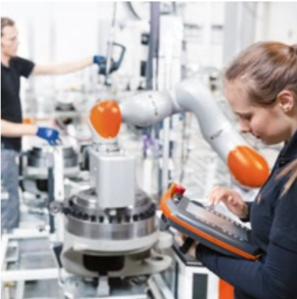
The HRC-capable LBR iiwa works hand in hand with humans and, as a result, is revolutionizing industrial production and manufacturing.
