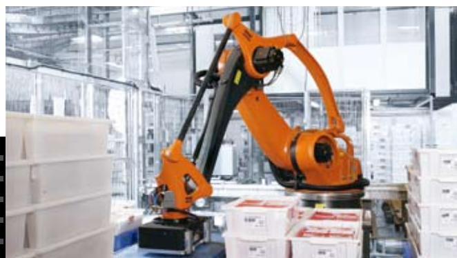
Fast, light, precise – and a great design: the use of carbon-fiber-reinforced components opens up many advantages.
