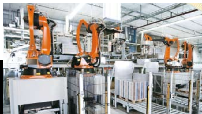
Whether mounted on the floor or on a pedestal (as seen here): with approx. 30 cycles per minute, the KR 100-2 PA and KR 180-2 PA excel all down the line.
